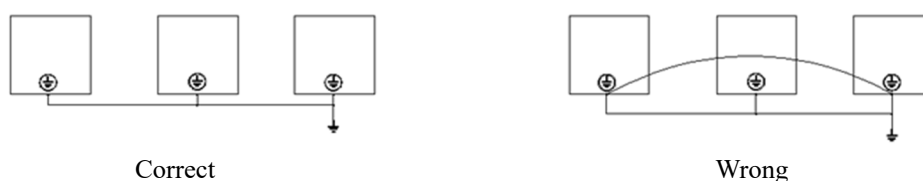
Figure 3-8 Grounding Wire Connection Sketch Map
