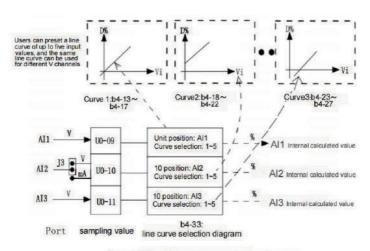
Figure 4-26 The Al signals correspond to the actual given
