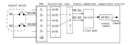
KOC550 series inverters provide a variety of terminal control methods, and the switch signal mode and function code can be determined through function code b4-11 b4-00 $\sim$  b4-07 determine the input port of start -stop control signal. For specific setting methods, please refer to b4-11, b4-00 $\sim$  b4-07, etc. A detailed explanation of energy codes.
