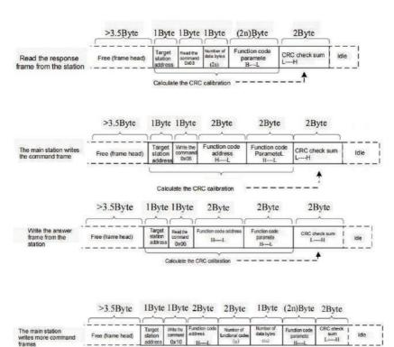
Multi-write is the same as multi-read, it can only operate up to 12 parameters continuously
