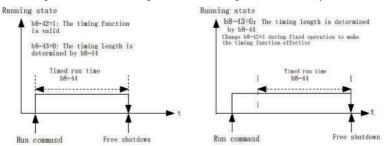
For the length of the timing time, the user is also provided with an available analog quantity (such as a potentiometer signal) for setting, please refer to b8-43 detailed description of the function code.
