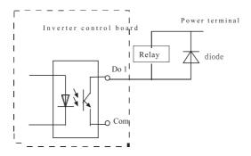
Figure 3-10 wiring diagram of digital output terminals
