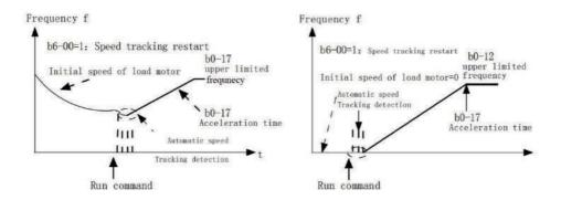
Figure 4-7 speed tracking restart mode
