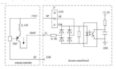
Figure 3-9 source connection mode
