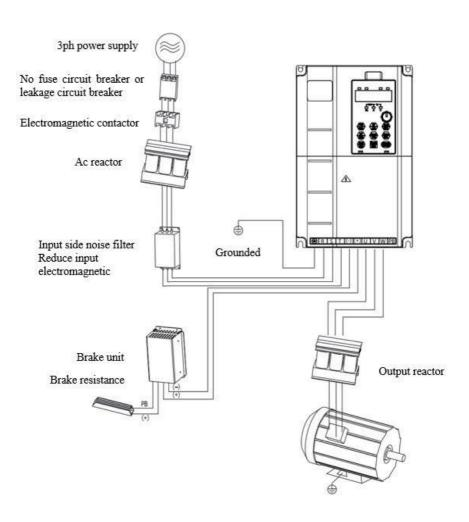
Inverter system configuration diagram
