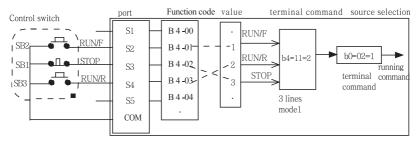
Figure 4-4 example of terminal start-stop control mode
