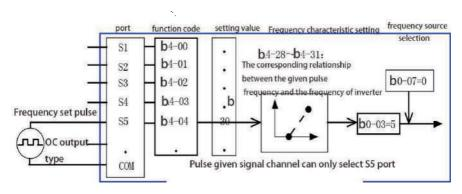
Figure 4-19 PULSE given frequency function code setting
