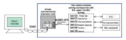
Figure 4-27 the use of inverter serial communication
