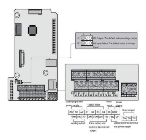
Figure 3- 2 KOC550 series control board diagram
