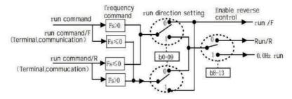
Figure 4-22 Setting the motor running direction
