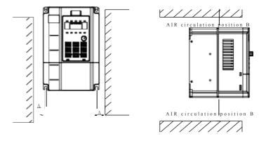
Figure 3-1 schematic diagram of inverter installation
