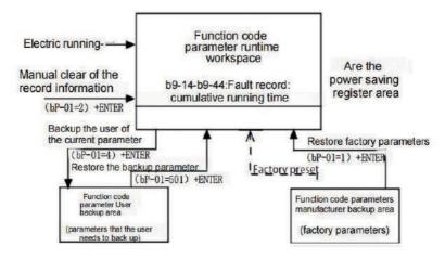
Figure 4-28 Parameter backup and recovery settings.
