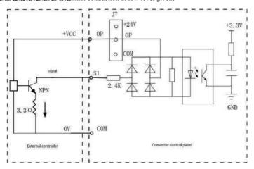
In this mode, the terminal is connected with a given low level (the optocoupler is turned on).
