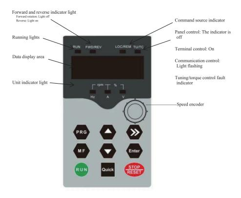
Figure 4-1 schematic diagram of the operation panel
