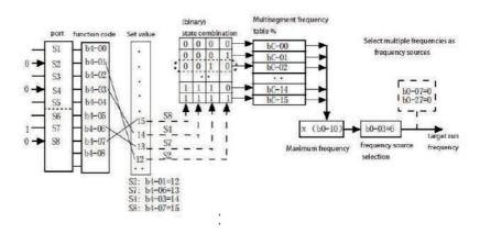
Figure 4-21 setting of multi-speed mode
