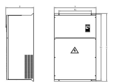
Figure KOC550 series high-performance vector inverter G22 $\sim$  G 400 kw sheet metal structure appearance and installation dimension drawing
