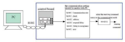
Figure 4-5 example of communication start-stop control mode
