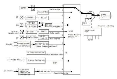
From the different frequency sources in the figure, it can be seen that the operating frequency of the inverter can be determined by the function code, and can also be adjusted manually in real time. It can also be set by analog quantity, or by multi-speed terminal command, or by external feedback signal, by the built-in PID the regulator is used for closed-loop adjustment; it can also be controlled by the host computer communication
