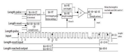
Figure 4-2 3 function code setting of fixed length control mod
