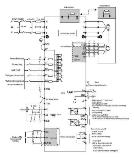
standard connecting wiring (3ph 380v)
